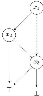
Dotted edges are used to indicate paths where the variable is false, while solid edges indicate paths where the variable is true.
