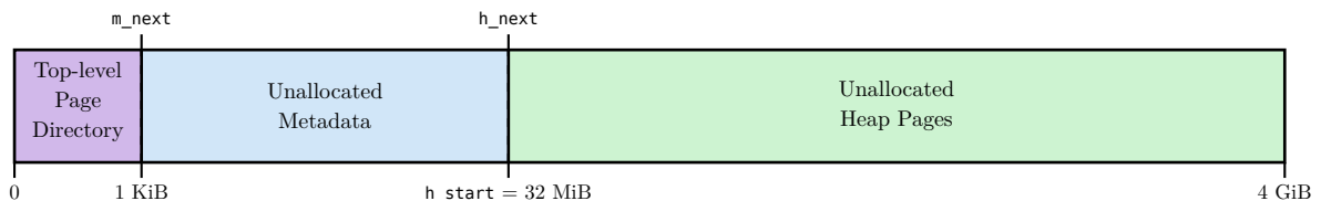
Figure 1: Physical memory layout at startup of the machine (not to scale)
